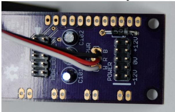
The fully assembled modules from Tsykron Labs have both power connectors installed, but this is DIY, so install what you need/want.
