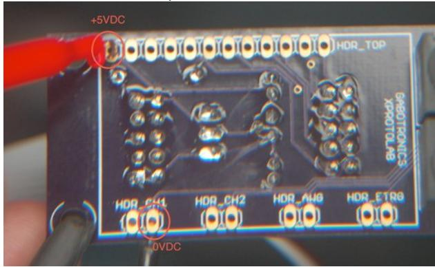
Then, check your voltmeter reading. You should read somewhere close to 5VDC. As shown in the picture below, 4.98VDC is close enough for rocket science, and synthie stuff.
