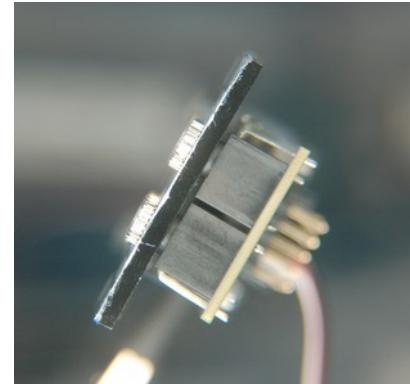
I6) The first step to soldering the rest of the TRACE module is to start with the Xprotolab module. With everything assembled, you can wiggle the Xprotolab module into place. Press the Xprotolab module against the back of the front panel until the the buttons are flush with the front of the front panel and the USB jack on the Xprotolab is flush against the back of the front panel. Once you have the Xprotolab module aligned, start by soldering every other pin on both sets of headers.
