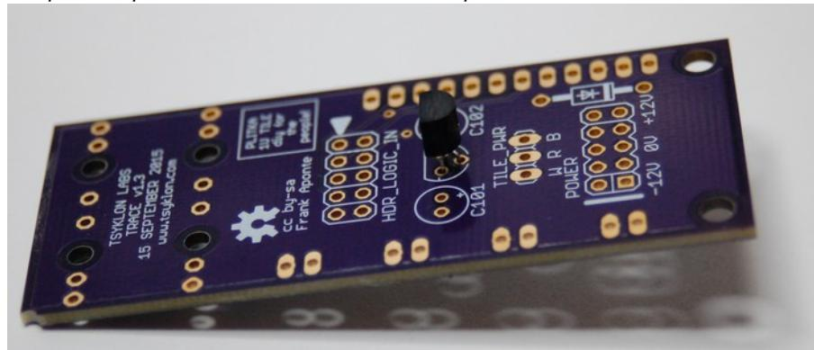
6) Next, install the reverse voltage protection Diode D101. Be sure to line up the silver stripe on the diode's Cathode with the silver stripe on the PCB silkscreen.
