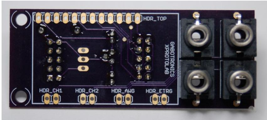
I4) Insert the Xprotolab module into the PCB. The I/O Jacks should be to your right with the Xprotolab buttons to the bottom.
