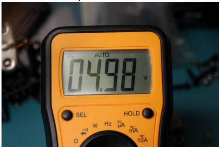
If your on-board power supply rings true, you are ready to proceed. If not, double check your solder joints, and check your work for shorts or open connections.
