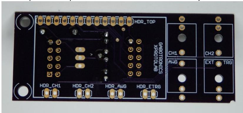
9) Solder the rest of the pins on both 2x5 pin headers. Some headers require more than a little heat to make the solder flow. This heat can soften the plastic that holds the header pins together and aligned. For this reason, I like to take a 2x5 ribbon cable connector and place it on the header pins to keep them aligned during the soldering process.
