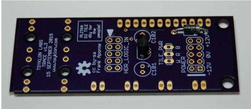
7) Install capacitors C101 and C102 into the PCB and solder. This style of capacitor, an Aluminum Electrolytic Capacitor, IS a polarized device - which means that its installation orientation DOES matter. Be sure to install the negative pin opposite the + marking on the PCB silkscreen.
