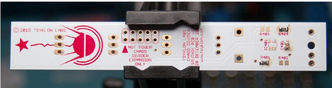
2-3) Install resistors R402 and R403 [2 x 24kΩ] onto the PCB and solder them in place:
