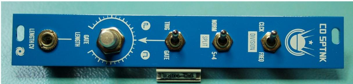
2-9) Perform your final flux clean up on the back of the PCB and install the knob onto VR\_GATE\_LEN:
