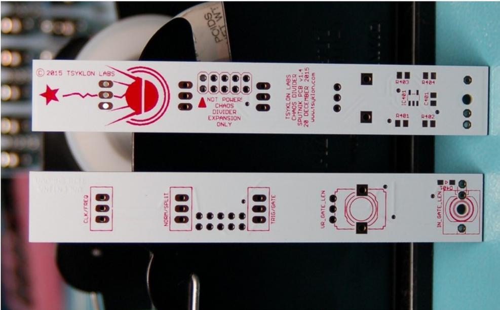
I-2) Next, we will inspect the Chaos Divider Sputnik Front Panel. Check for chips or flakes in the powder coated panel as well as any issues with the screen printing. It should look like this:
