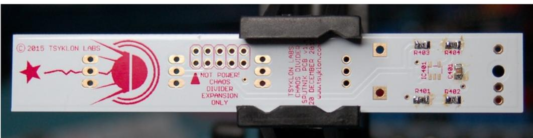
2-4) Now that you have warmed up on the easy SMD components, install IC401 [1 x TLV237IDBVS] onto the PCB and solder it in place:
