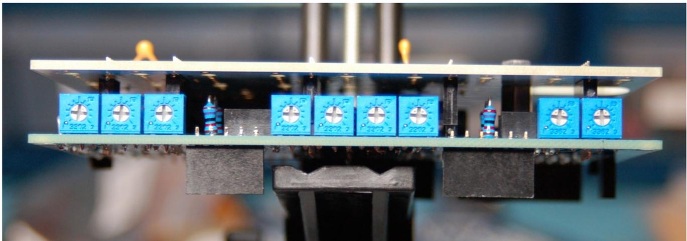
If you want to set the output amplitudes more precisely, try this – flip the **NORM/INV** toggle switch “up” to the inverted setting. Then, when you either press and hold the **RESET** pushbutton or inject a 5VDC signal into the **RESET** input jack, all of the outputs will remain on. Then, set the trim pots while monitoring the voltage for each output jack with a meter or scope.
