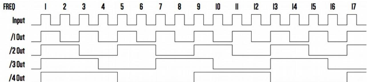
These two types of clock modulation are the basic modulation functions of the Tsyklon Labs Chaos Divider. The rest of the features available in the Chaos Divider are extensions of these functions.
